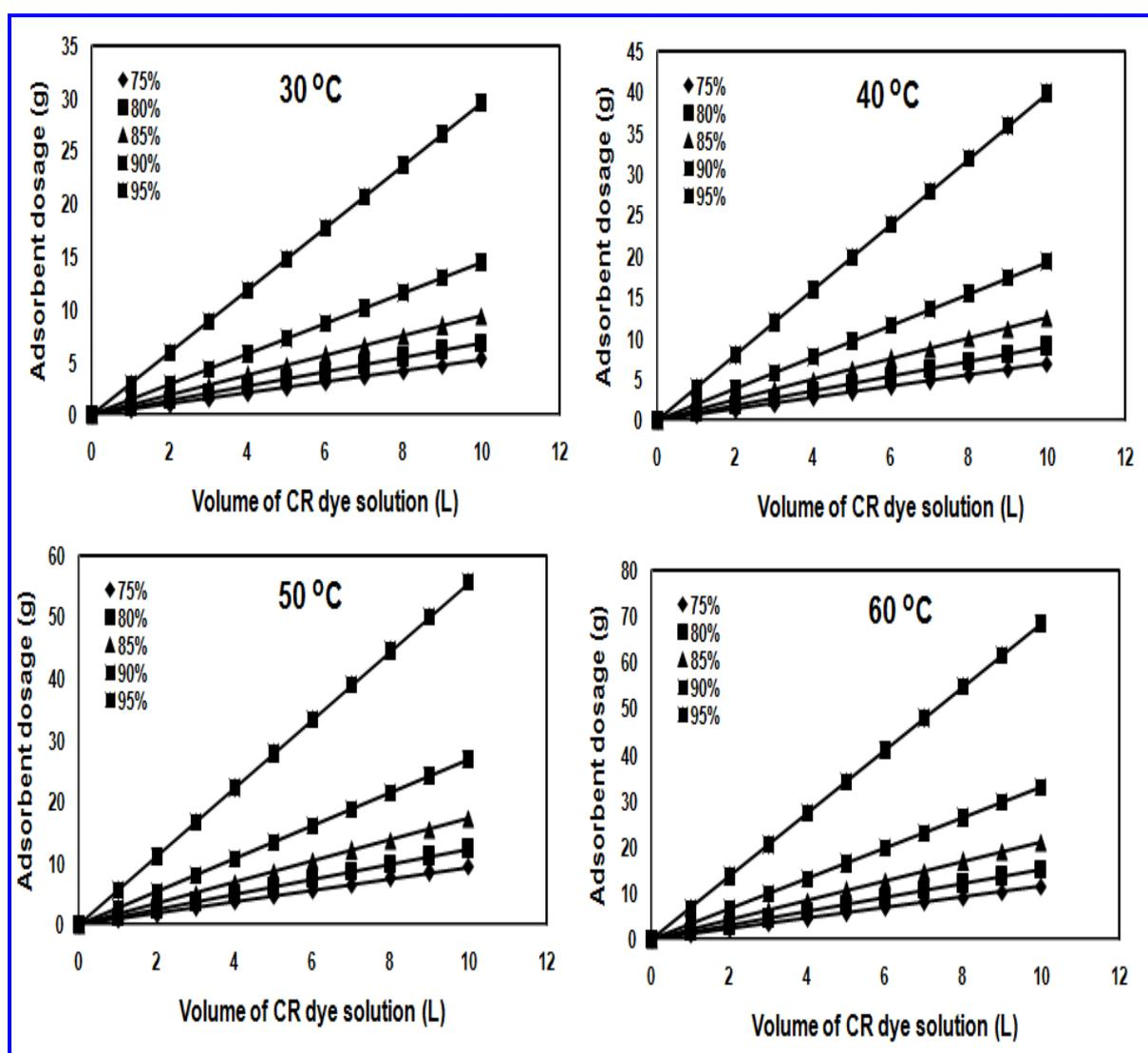
Fig. 11: Adsorber design results for the removal of CR dye by NiO-CNC
