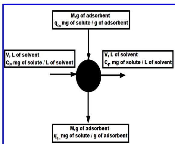
**Fig. 10: Single-stage batch adsorber design**
